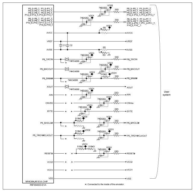
Figure 7.1 Connection diagram
